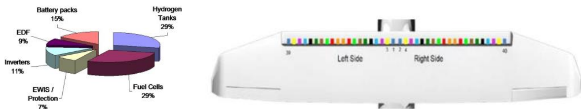
Figure 38: Left: Estimated MTOW breakdown for the high-wing concept aircraft. Right: Fuel cell/battery clusters and corresponding EDFs (one color for each cluster).
